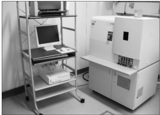
Fig.9 Example analyzer (ICP-AES) for environmental control substances
