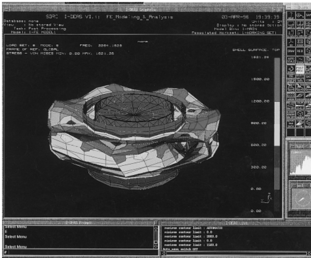
Fig.3 Vibration mode and stress distribution on the runner
