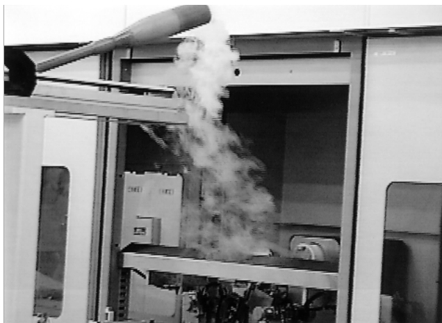
Fig.3 Verification of air flow with a visualization system
