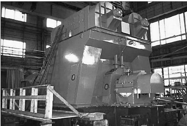
Fig.12 Example of synchronous electric motors for main rolling mill
