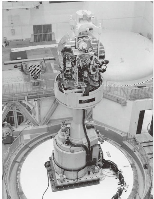
Fig.6 Heat-resistant restraint mechanism of the core for very high temperature gas reactor (VHTR)
