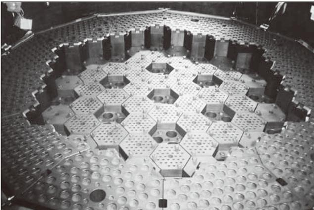
device for conducting creep testing inside the HTTR core<sup>(6)</sup>.
