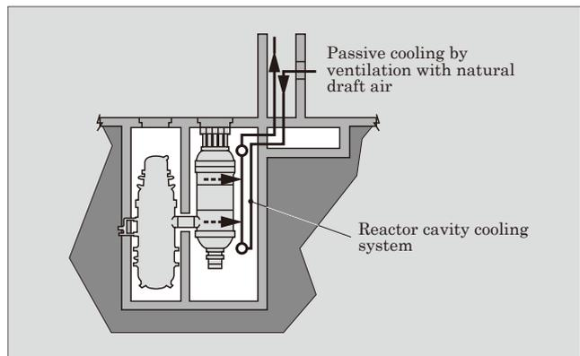
temperature of a HTGR during normal operation has sufficient margin to the limiting temperature under accident conditions, and therefore, at the time of an accident, even without an emergency shutdown action of the control rod, the reactor will be shut down passively due to the negative reactivity feedback.
