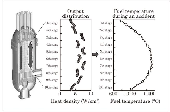
Fig.8 Example of analysis result of heat removal from reactor by natural cooling
