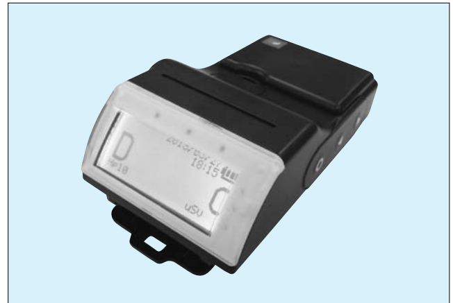
Fig.16 “NRF51” new electronic personal dosimeter
