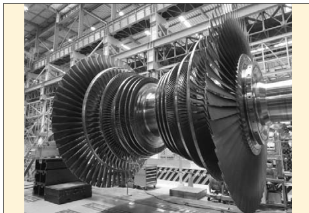
Fig.4 Low-pressure turbine rotor
