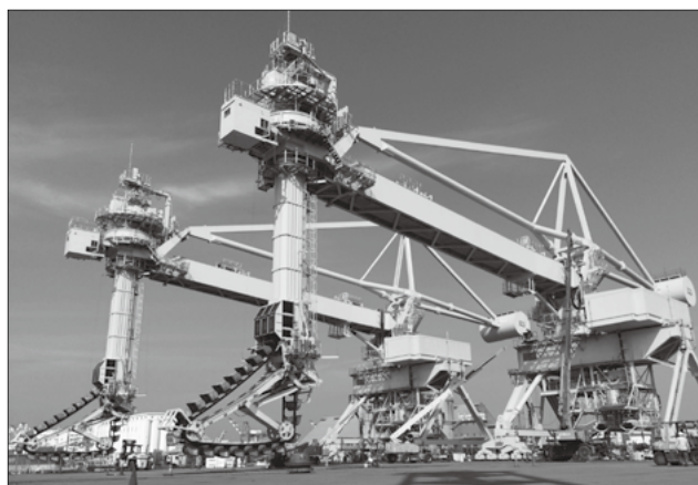
Fig.8 Overall view of continuous unloaders
