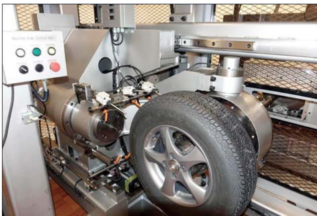
Fig.4 WLTP compliant tire testing machine
