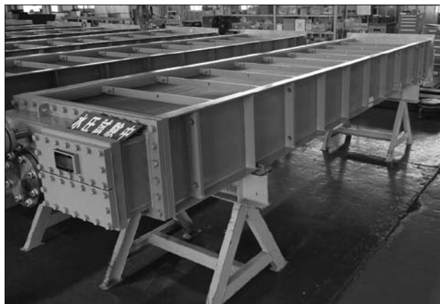
Fig.5 Hydraulic pressure test on air cooler
