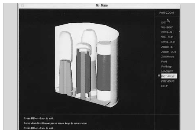
Fig.5 3-D model for electric field analysis (cable sealing end, lightning arrester)
