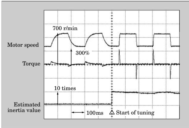
forms. When the total inertia value is 10 times the motor inertia, the initial value of inertia is estimated as unity. When real-time auto-tuning is started at point  $\triangle$  mark, the inertia is instantaneously estimated
