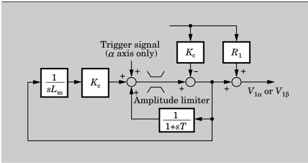
of appropriate positive feedback through control of the microprocessor and the inverter, self-excited oscillation near the synchronous frequency and speed estimation is possible. Figure 6 shows a control block diagram (stationary frame  $\alpha, \beta$  axis) for self-excited oscillation. With the control, the inverter can excite the induction motor near the synchronous speed regardless of the motor speed by supplying the reactive power needed by the induction motor.
