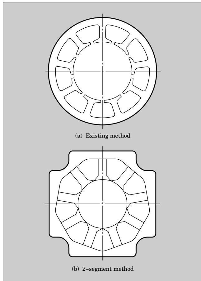
wound, is attached to each tooth. This assembly is fitted into a ring yoke, forming the completed armature core. The fitting clearance at each tooth between outer and inner cores must be maintained as even as possible to obtain better characteristics.
