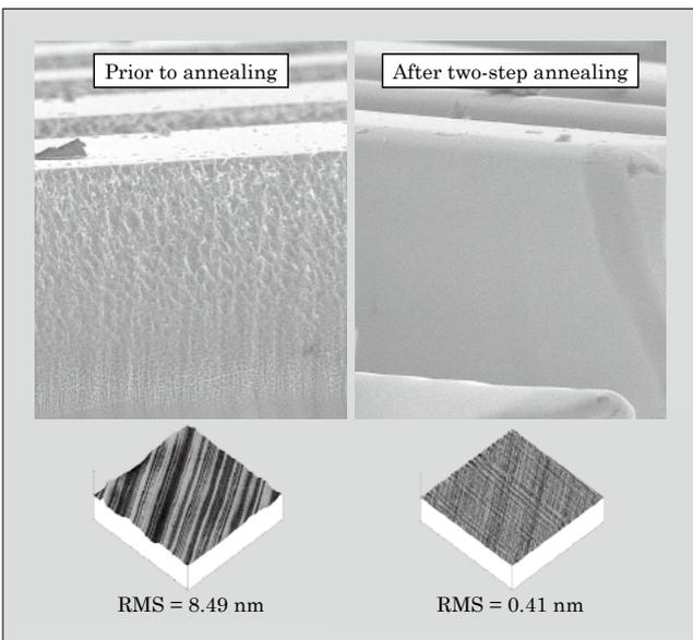
trench sidewall of a sample was evaluated both before and after performing two-step annealing with  $\text{SiH}_4/\text{Ar}$  and  $\text{H}_2$ , and the results are shown in Fig. 8.
