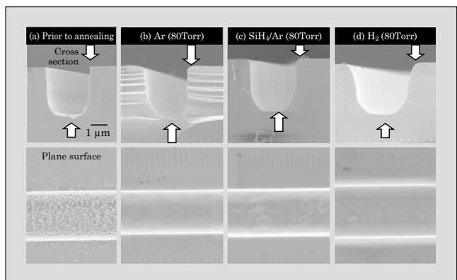
Fig.4 Temperature dependency of SiC trench shape with annealing in SiH<sub>4</sub>/Ar atmosphere
