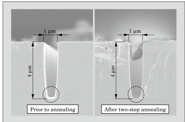
able to verify that the two-step annealing process resulted in extremely smooth trench sidewalls.
