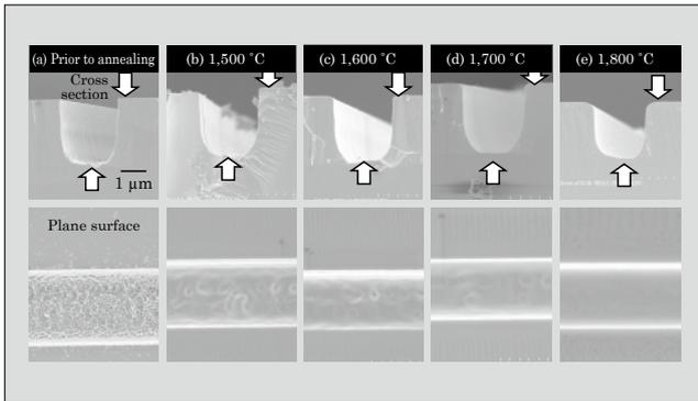
Fig.5 Temperature dependency of SiC trench shape with annealing in H<sub>2</sub> atmosphere
