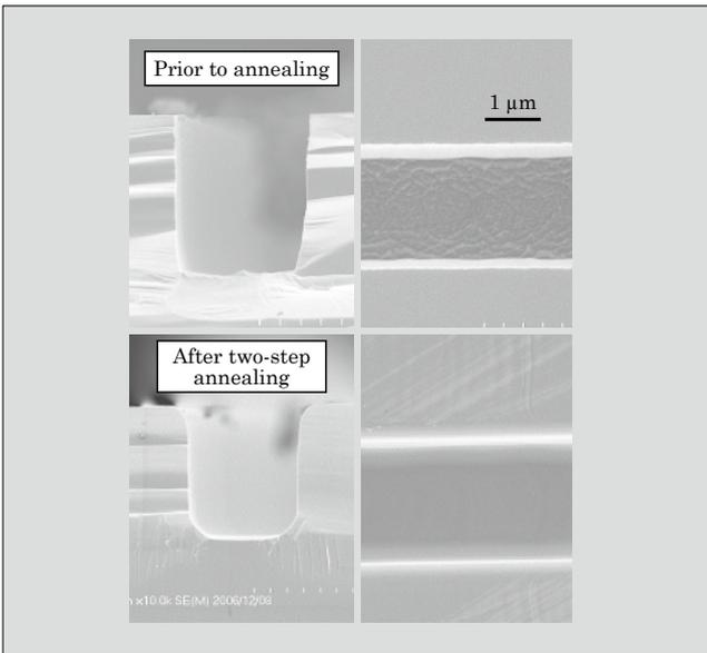
Fig.8 Improvement in trench sidewall due to two-step annealing
