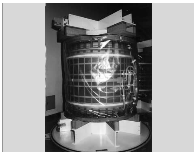
Fig.3 Winding assembly packaged with film
