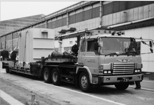
Fig.6 Testing of the core component transportation
