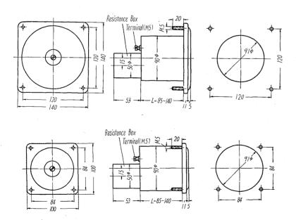
Fig. 2. Outline Dimensions and Drilling Plans of Wide Angle type Instruments
