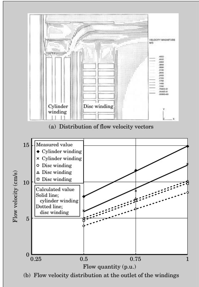
and momentum. The software performs a steady state analysis using a turbulent flow model.
