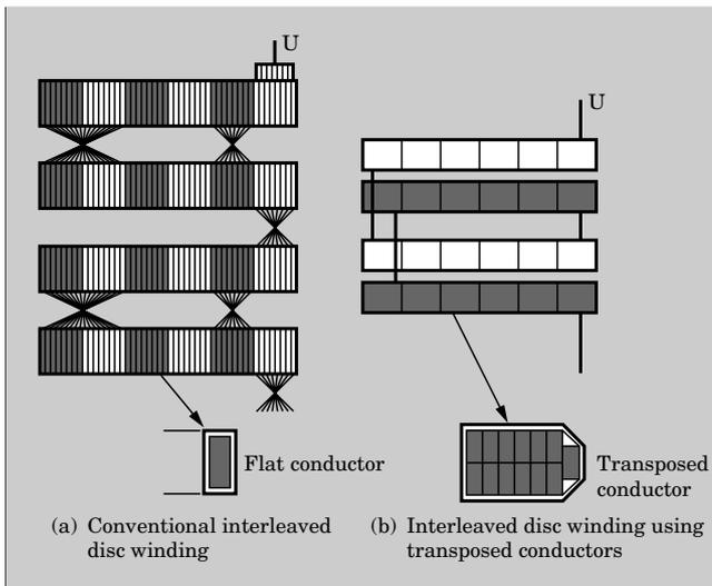
between coils that are axially arranged. Figure 1 compares coil compositions and conductor connections of the interleaved windings.
