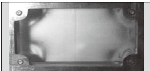
out around the screw locations, but despite using a flat fin, the spreading of thermal grease in the center area was poor. To investigate the cause, a photoelastic camera was used to measure the distribution of stress generated between the IGBT module and fin when the IGBT module and fin mounting screws are tightened. An FEM (finite element method) analysis was also performed at the same time.
