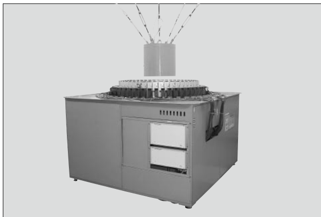
Fig.5 Photograph of gamma-ray calibrator (middle level)
