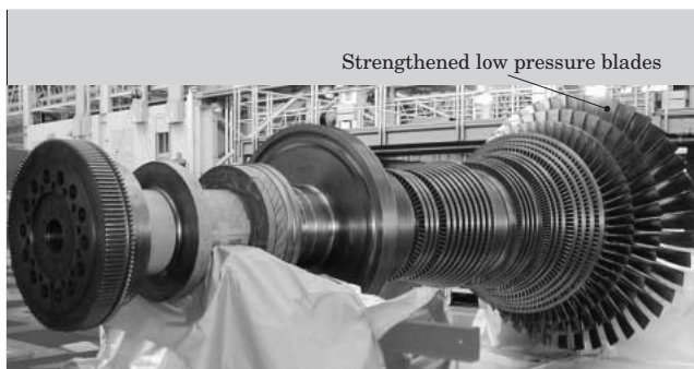
Fig.14 Strengthened low pressure blades
