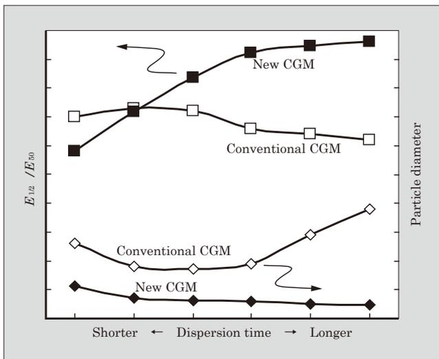
teristics, and meets its customers' demands for image gradations and other properties. It also develops CGM dispersion techniques and is improving sensitivity characteristics by adjusting the CGM particle diameter (Fig. 6).
