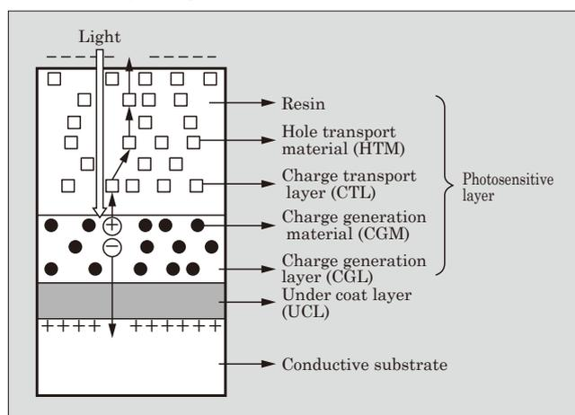
Fig.2 Layer Composition and Materials of Positive Charge Multilayer Organic Photoconductors
