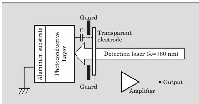
Fig.2 Relationship between Surface Potential and Induced Current
