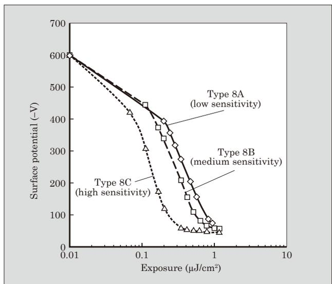
resolution can be met by developing a CTM with low horizontal charge diffusion. The fine line definition reduces the amount of toner consumed, which reduces printing costs.
