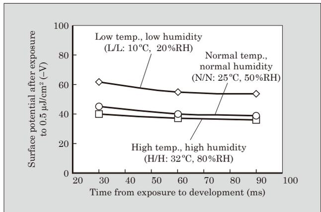
Fig.5 Photo-induced Discharge of Negative Charge OPCs
