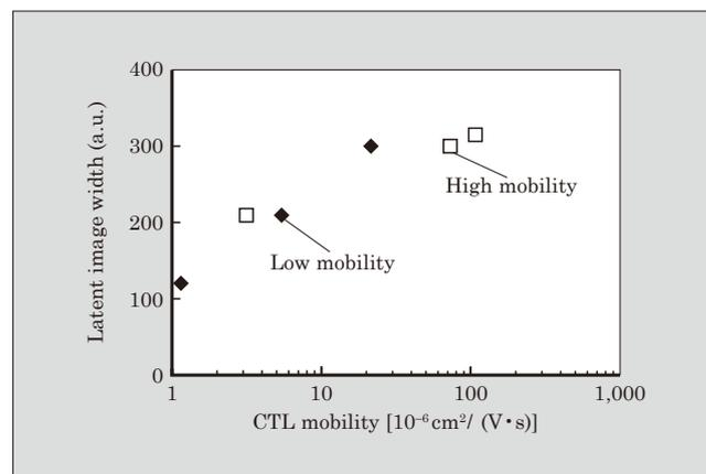
Fig.7 Dependence of Latent Image Depth on Mobility
