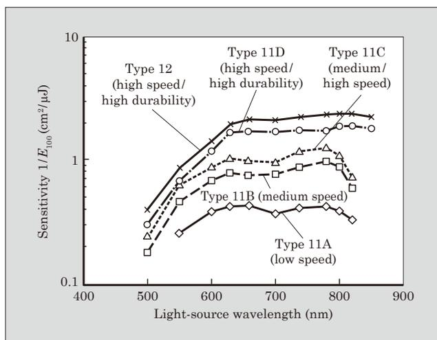
Fig.9 Photo-induced Discharge (PIDC) of Positive Charge OPCs
