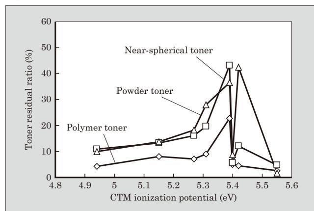
This makes the toner adhere strongly to the OPC surface (“filming”), and low-filming performance is therefore required. Fuji Electric develops and employs methods to evaluate the adhesive strength of toner using the toner residual ratio<sup>(1)</sup>. Figure 7 shows the CTM ionization potential and toner residual ratio of each toner. Fuji Electric is developing the optimum OPCs for each type of toner.
