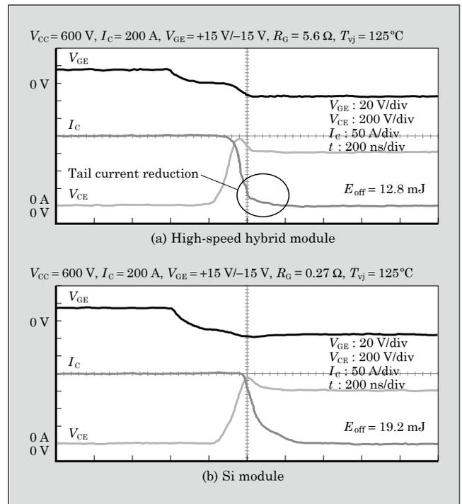
Fig.4 Turn-off waveforms
