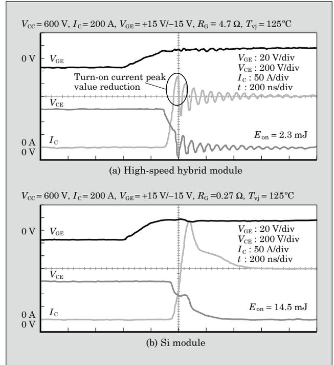
Fig.3 Turn-on waveforms
