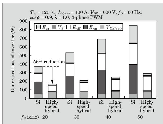
Fig.1 Inverter generated loss simulation results
