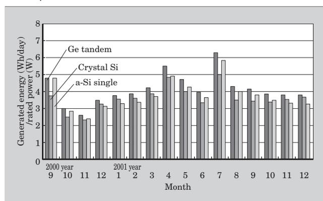
Available energy on AC side can be obtained by multiplying by the inverter efficiency (0.9).
