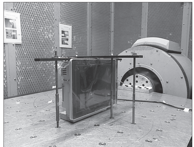
Fig.5 Acceleration resistance test circumstance
