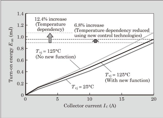
Fig.7 Collector current dependency of the turn-on energy
