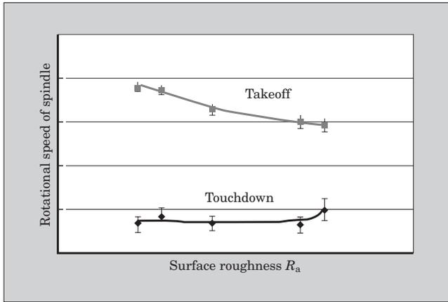
Fig.3 LUL durability in a reduced pressure environment
