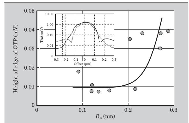
Fig.4 ByER dependency on surface roughness ( $R_a$ )
