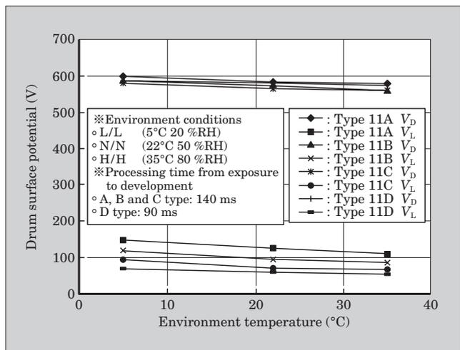
Table 4 Variation in characteristics due to environmental testing of positively charged OPCs
