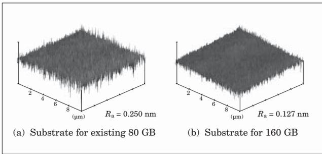
Fig.3 Surface defects of a polished aluminum substrate
