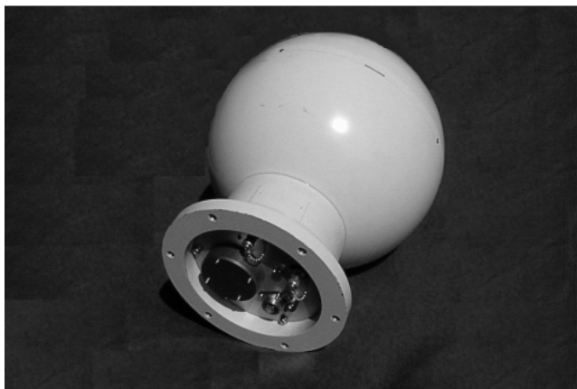
Fig.3 Spherical ionization chamber detector
