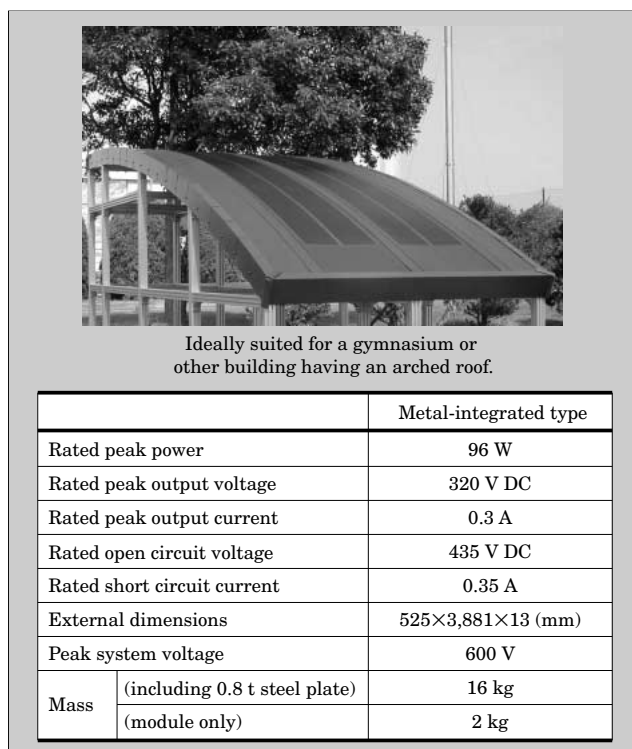
Fig.5 Metal-integrated PV module and its specifications
