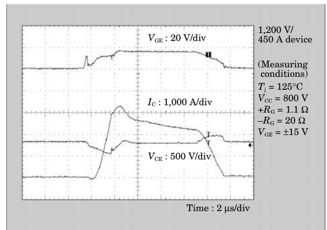
Fig.5 Comparison of IGBT turn-on waveforms for U-FWD and conventional FWD
