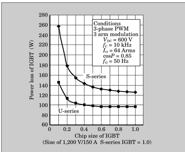
Fig.7 Comparison of output characteristics of IGBT
