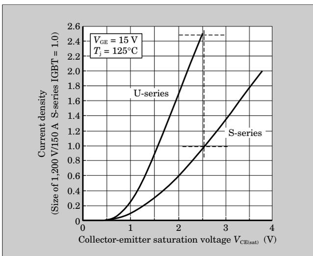
characteristic was improved as shown on Fig. 7. This improvement was realized because of the fact that the saturation voltage will not be increased by the increase in current density.
