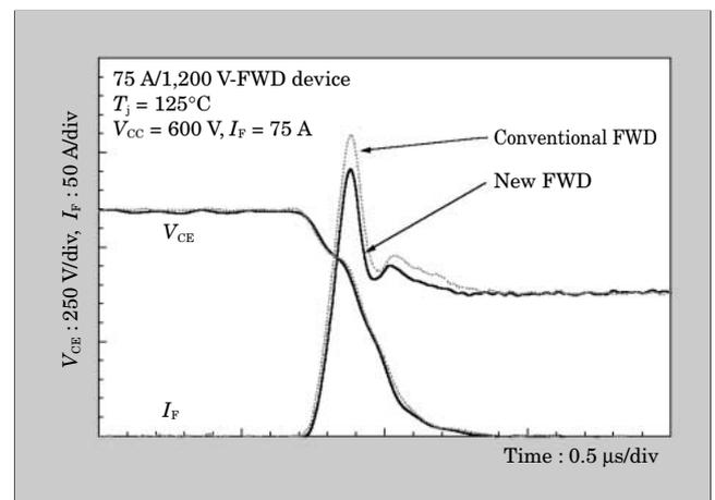
as shown on Fig. 5. As a result, turn-on power loss was reduced.
