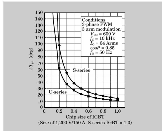
Fig.9 FEM analysis results of chip temperature rise of IGBT
