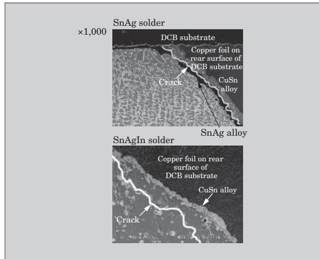
Fig.5 Results of tensile test for SnAg and SnAgIn solder at room temperature
