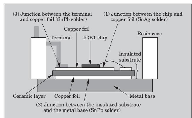
foil. Lead-free solder has been used in location (1) since 1998, and the ability to withstand power cycles of this lead-free solder has been successfully improved. Therefore, our new development aimed to make locations (2) and (3) lead free.
