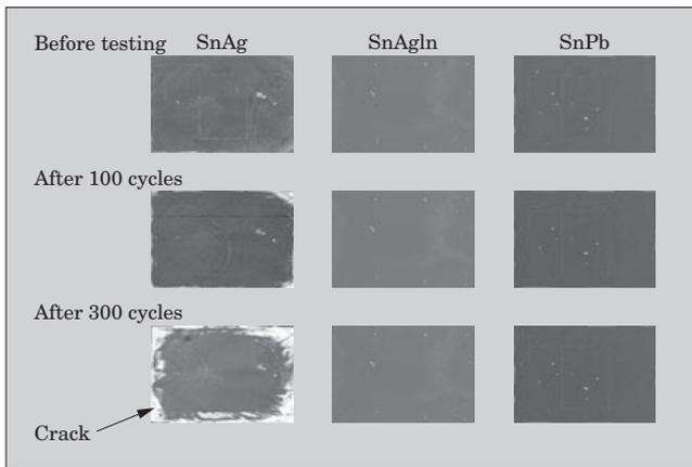
Fig.3 Results of simulated thermal stress of solder between insulated substrate and metal base (FEM analysis results)
