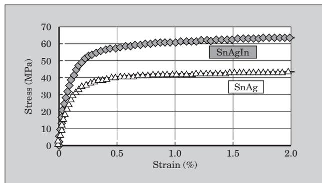
Based on the above results, the addition of In to the SnAgIn solder results in: ① suppression of the formation of a SnAg alloy layer, resulting in a change from fracturing at the alloy boundary to fracturing of the bulk solder material, ② an approximate 1.5 times improvement in bulk strength, and ③ particles that do not become coarser during thermal cycling tests. These factors are thought to improve the ability to withstand the thermal cycling tests.
