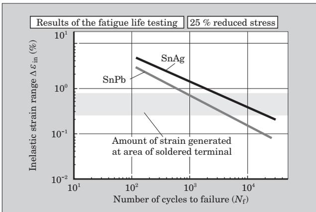
results of Fig. 6 is also shown. For withstanding generated strain, it can be seen that SnAg solder has the same or longer lifespan than SnPb solder.
