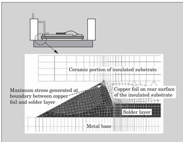
underneath the IGBT module during a thermal cycle test. In this drawing, the maximum stress is generated near the boundary between copper foil on the rear surface of the insulated substrate and the solder layer.
